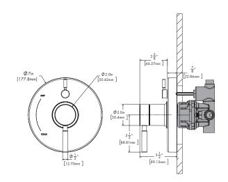
VALVE MOUNTING IS SHOWN FOR REFERENCE ONLY. VALVE IS NOT INCLUDED WITH CPT-1401/CPT-1401-KN
